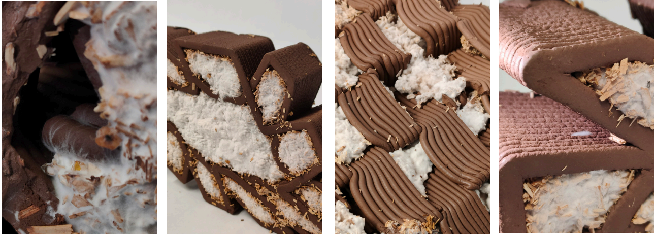
Mycelium growth within non-fibrous fired clay and mycelium
