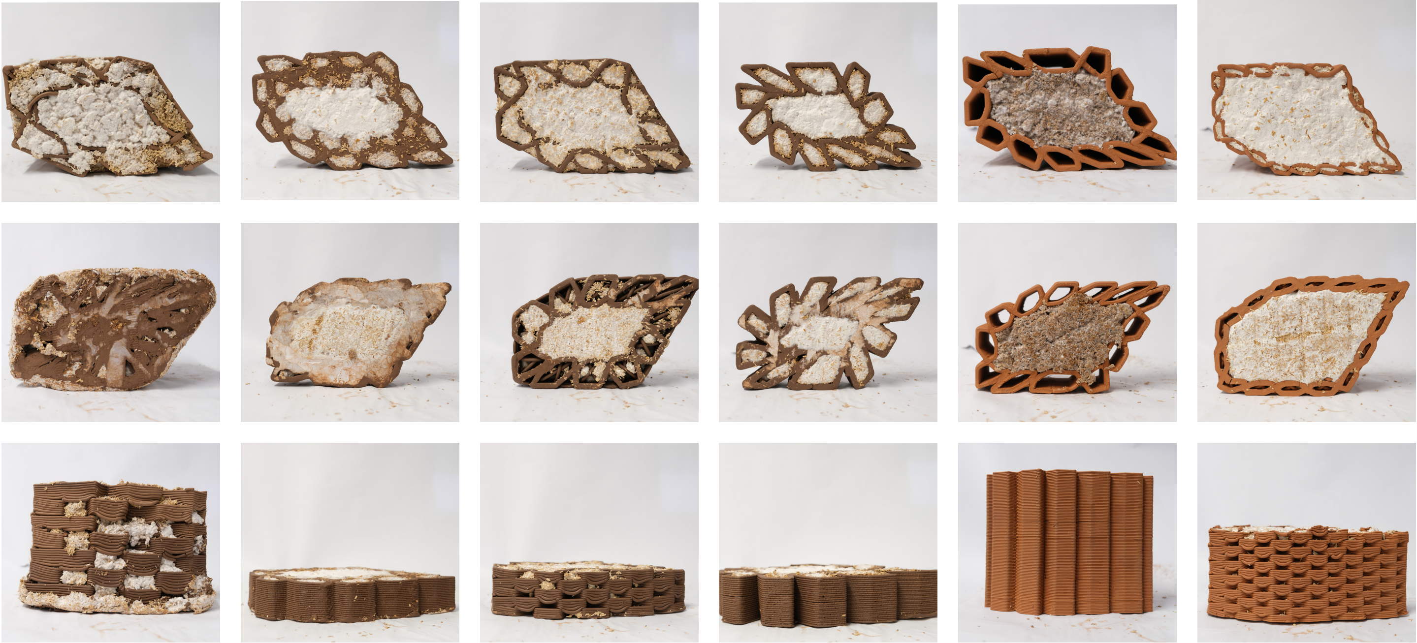
Iterations of grown modules with varied height and internal patterns
