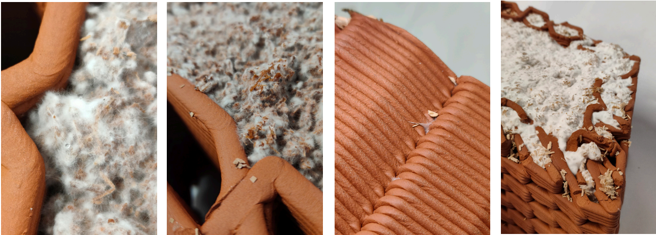
Mycelium growth within non-fibrous fired clay and mycelium
